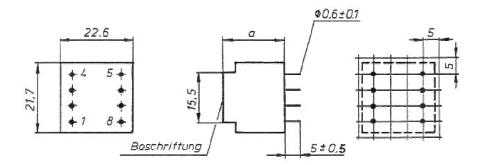
Dimensions with no indication of tolerances: +/- 0.3 mm.
